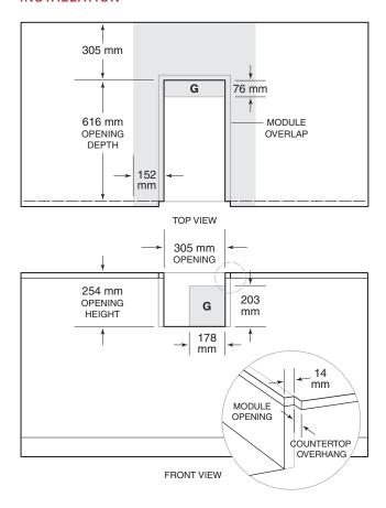
NOTE: Shaded area above counter top indicates minimum clearance to combustible surfaces, combustible materials cannot be located within this area. An insulating liner is not required for the ICBBM13.
