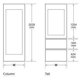
Typical panel dimensions are based on a 2134 mm finished height with a 102 mm toe kick and 3 mm reveals. Panel dimensions must be adjusted accordingly for all other installations. Refer to the illustration for panel heights and the chart below for panel widths.
