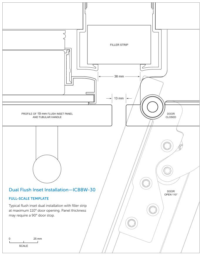
Dual flush inset installation (top view)
