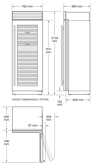
Dimensions are based on the stainless steel model. For flush inset applications, add 13 mm to the door clearance dimensions.
