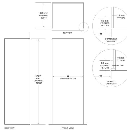
NOTE: 89 mm finished returns will be visible and should be finished to match cabinetry. Shaded line represents profile of unit.
