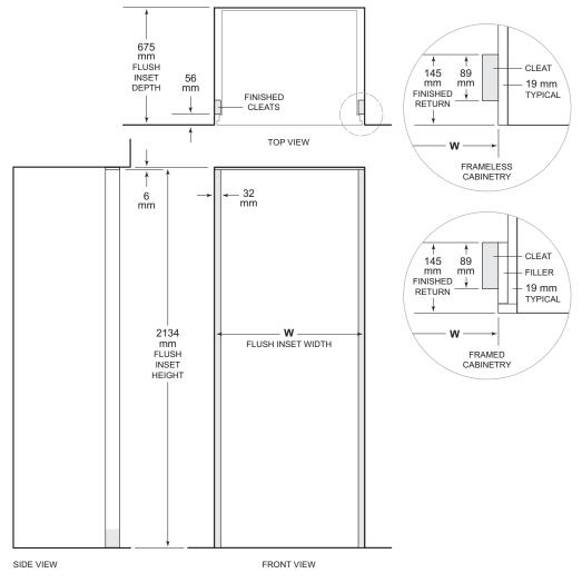
NOTE: 89 mm finished returns and shaded areas will be visible and should be finished to match cabinetry. Shaded line represents profile of unit with 19 mm panel.
