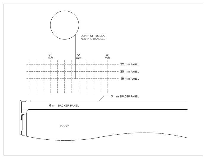
Overlay and flush inset panel thickness
