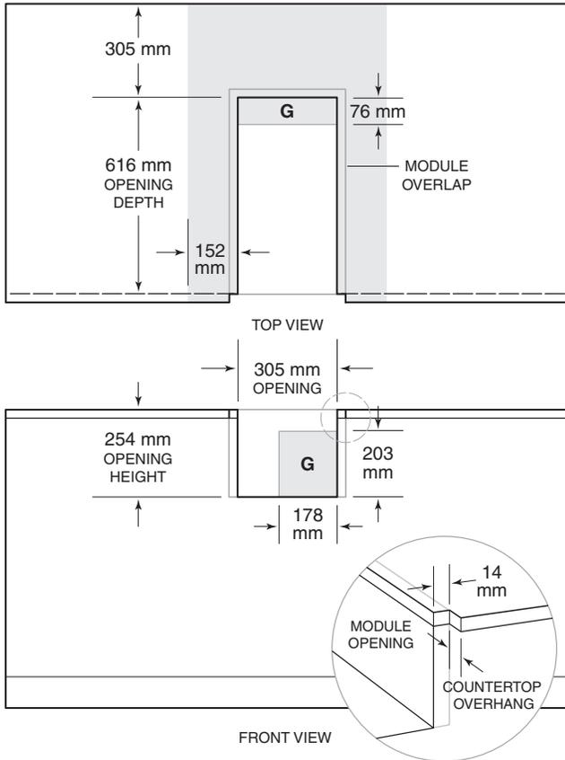
*NOTE: Shaded area above counter top indicates minimum clearance to combustible surfaces, combustible materials cannot be located within this area. An insulating liner is not required for the ICBBM13.*
