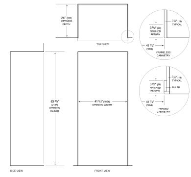
$NOTE: 3^{1}/z^{*}$  (89) finished returns will be visible and should be finished to match cabinetry Shaded line represents profile of unit.
