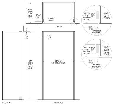
NOTE: 31/2" (89) finished returns and shaded areas will be visible and should be finished to match cabinets.
