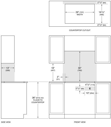
NOTE: Shaded area above countertop indicates minimum clearance to combustible surfaces, combustible materials cannot be located within this area. Electrical supply location only applies to installations with built-in oven.
